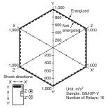
Conditions: Shock is applied in ±x, ±y, ±z directions three times each with and without energizing the relays to check the number of contact malfunctions
