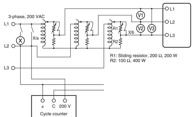
**Q** **Checking the Phase Sequence and Phase Loss Operation**
