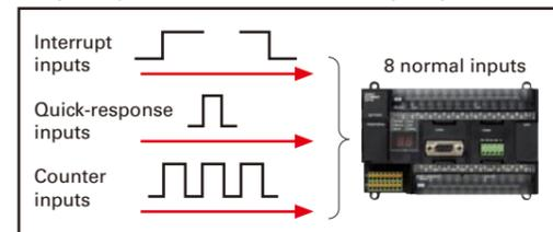
The normal inputs can be set in the PLC Setup as interrupt, quick-response, or counter inputs. (There are 8 normal inputs for the CP1H-X/XA, 6 for the CP1H-Y, 6 for the CP1L with 20, 30, or 40 points, and 4 for the CP1L with 14 points.)
