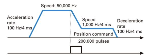
Interrupt input signal 00 (Input word 0, bit 00)
