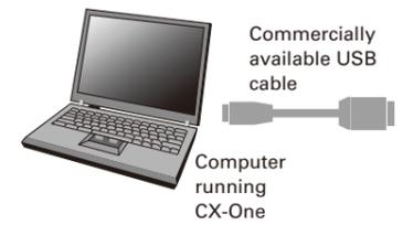
The built-in USB port lets you connect to a personal computer using a general-purpose cable.
