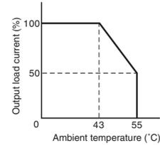
When using the CP1W-32ER, do not allow more than 24 outputs to be ON simultaneously regardless of the ambient temperature.
