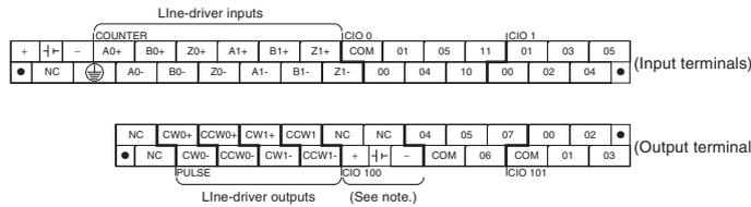
Note: Supply 24 VDC to the bottom 24 VDC input terminals when using bits 04 to 07 of output word CIO 100.
