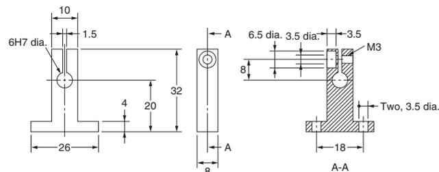
Tightening torque: 0.6 to 0.8 N·m (M3 screws)
