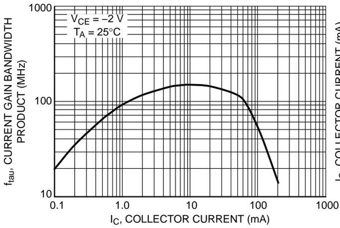
Figure 7. Current Gain Bandwidth Product vs. Collector Current
