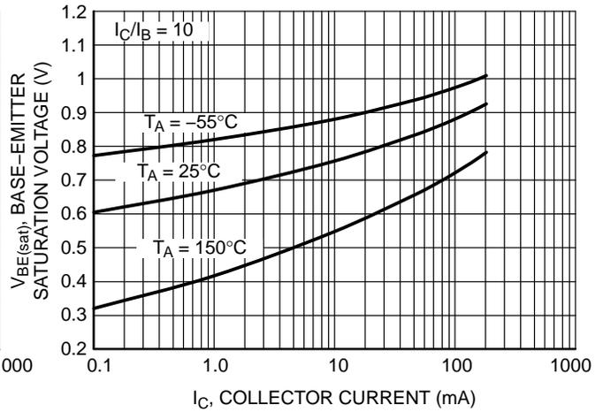
Figure 2. Base-Emitter Saturation Voltage vs. Collector Current
