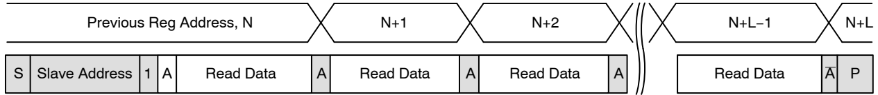
Figure 12. Sequential READ, Start from Current Location
