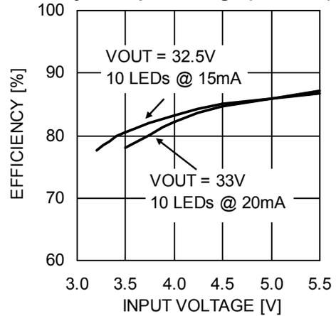
**Power-up with 10 LEDs at 20mA**
