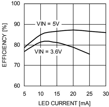
**Efficiency vs. Input Voltage (10 LEDs)**
