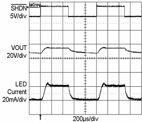
**Figure 1. Switching Waveform with 1kHz PWM on  $\overline{\text{SHDN}}$**
