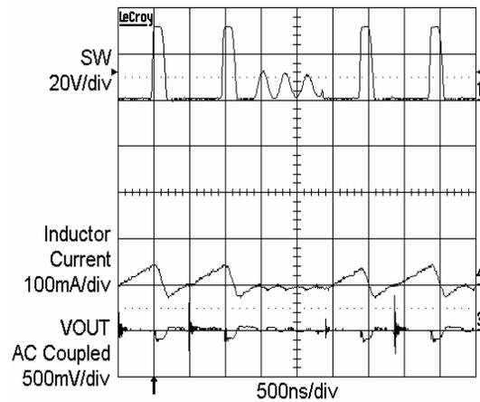
Switching Waveform VIN = 5.0V, I<sub>LED</sub> = 1.5mA
