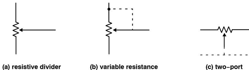
Figure 5. Potentiometer Configuration
