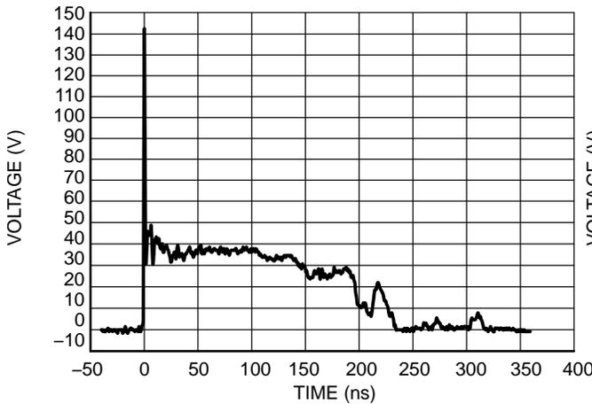
Figure 3. IEC61000-4-2 +8 kV Contact ESD Clamping Voltage
