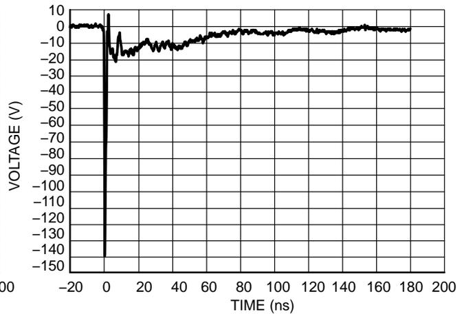
Figure 4. IEC61000-4-2 -8 kV Contact ESD Clamping Voltage
