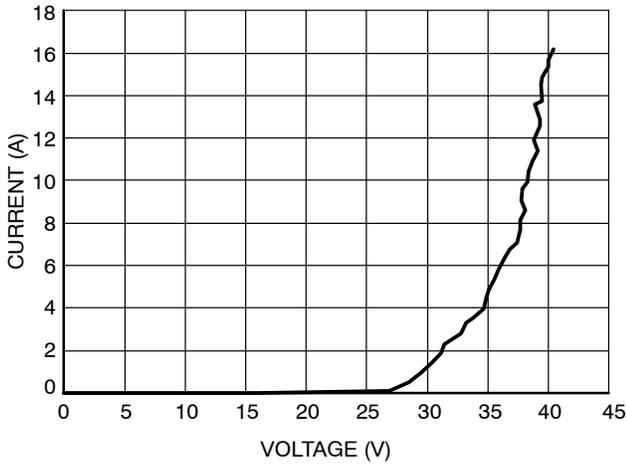
**Figure 5. Typical Positive TLP IV Curve**
