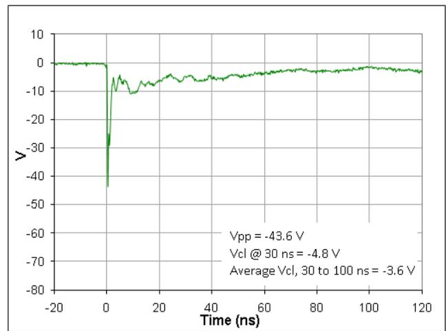
**Figure 6. ESD Clamping Voltage Screenshot
