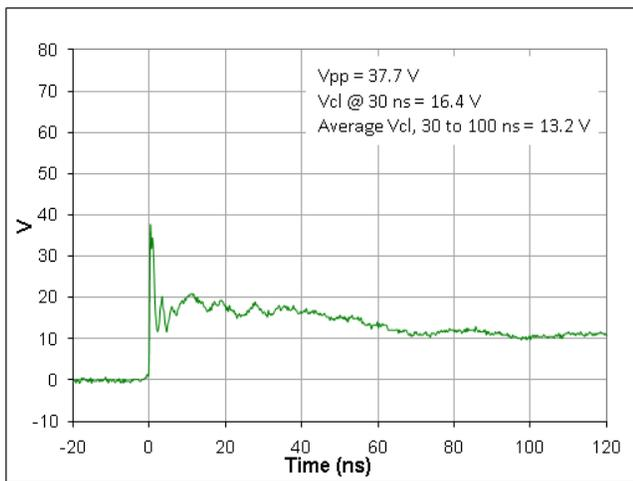
**Figure 5. ESD Clamping Voltage Screenshot
