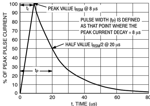
Figure 9. 8 x 20 μs Pulse Waveform
