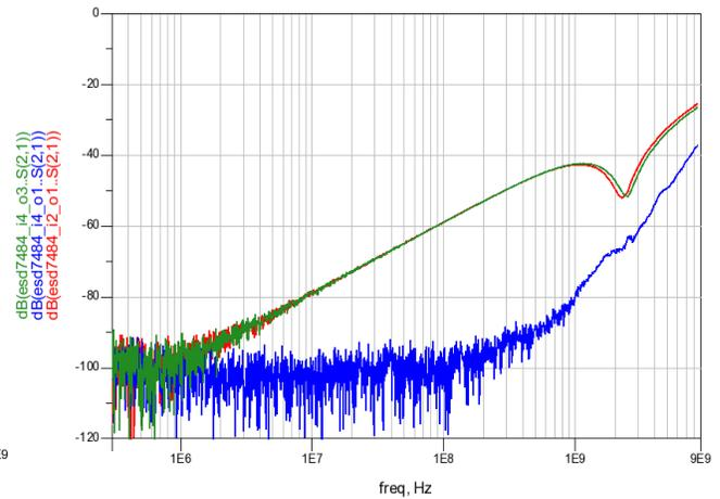
**Figure 4. Crosstalk Measurements**
