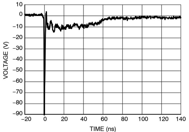
Figure 2. IEC61000-4-2 -8 kV Contact Clamping Voltage
