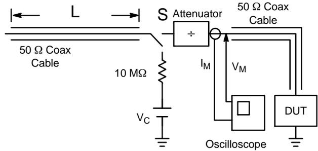
Figure 12. Simplified Schematic of a Typical TLP System
