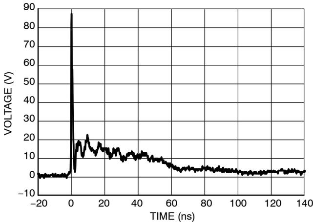
Figure 1. IEC61000-4-2 +8 kV Contact ESD Clamping Voltage
