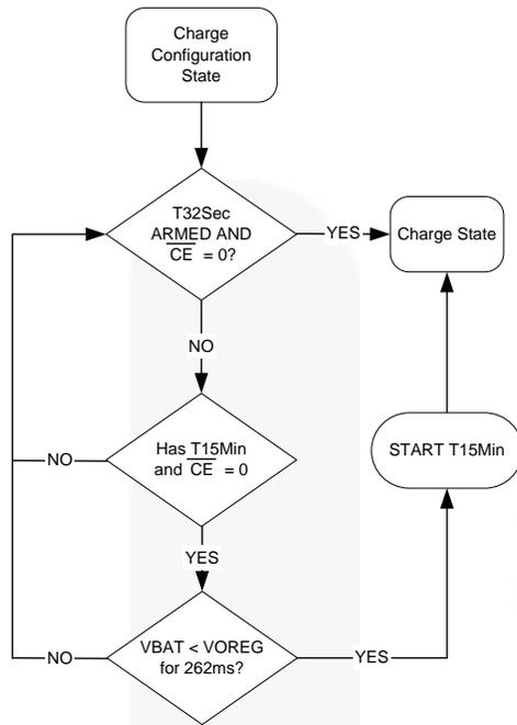
Figure 39. Charge Configuration
