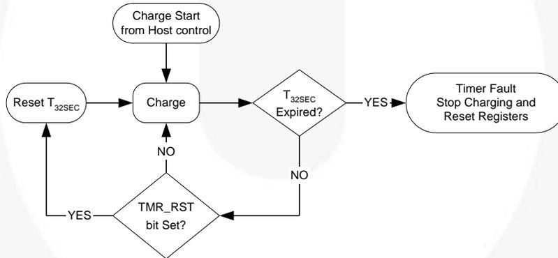
Figure 42. Timer Flow Chart for FAN5401, FAN5404
