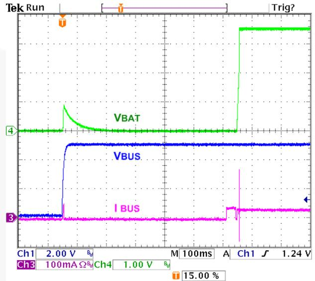
**Figure 18. No Battery at  $V_{BUS}$  Power-up; FAN5402, FAN5405**
