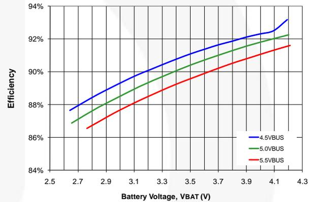
**Figure 10. Charger Efficiency vs.  $V_{BUS}$ ,  $I_{INLIM}=500\text{ mA}$**
