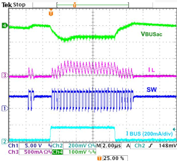
Figure 33. Load Transient, 5-155-5 mA,  $t_R=t_F=100\text{ ns}$
