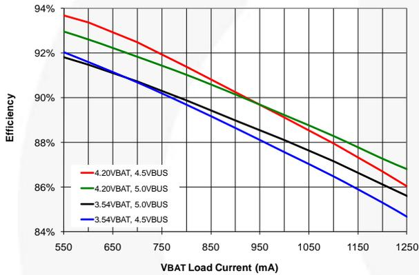
**Figure 9. Charger Efficiency, No  $I_{INLIM}$ ,  $I_{CHARGE}=1,250\text{ mA}$**
