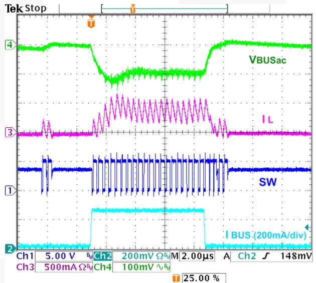
Figure 34. Load Transient, 5-255-5 mA,  $t_R=t_F=100\text{ ns}$
