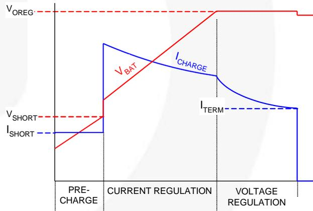
Figure 36. Charge Curve, I<sub>INLIM</sub> Limits I<sub>CHARGE</sub>
