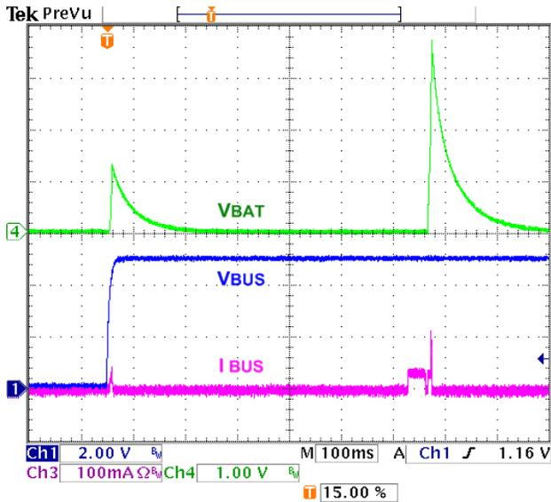
**Figure 17. No Battery at  $V_{BUS}$  Power-up; FAN5400, FAN5403**
