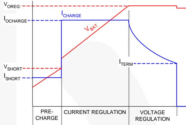
Figure 35. Charge Curve, I<sub>CHARGE</sub> Not Limited by I<sub>INLIM</sub>
