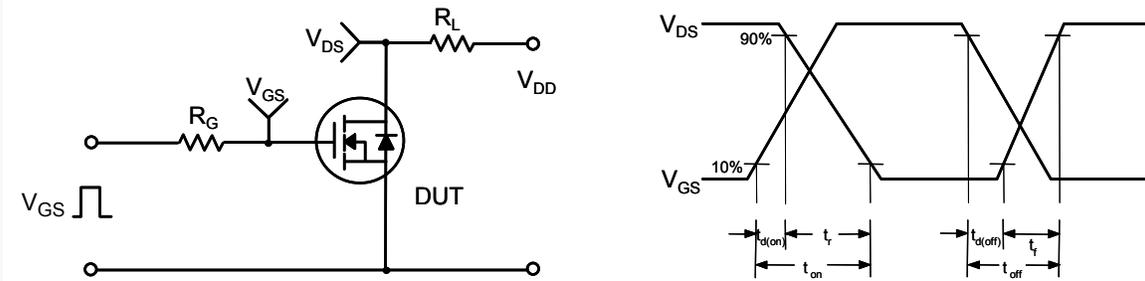
**Figure 14. Resistive Switching Test Circuit & Waveforms**
