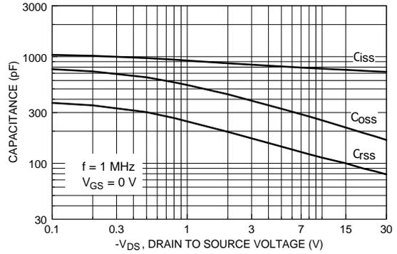
Figure 8. Capacitance Characteristics.
