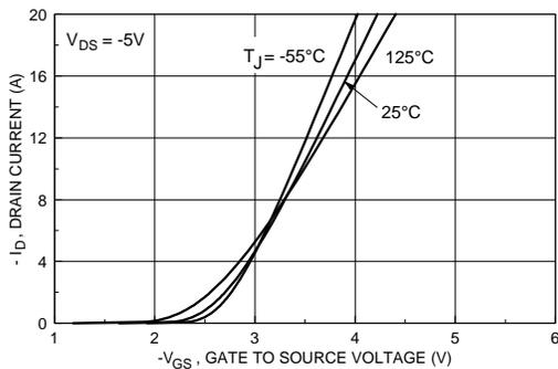
Figure 5. Transfer Characteristics.
