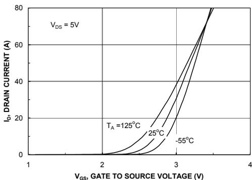
Figure 5. Transfer Characteristics
