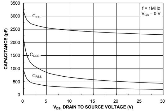
Figure 8. Capacitance Characteristics
