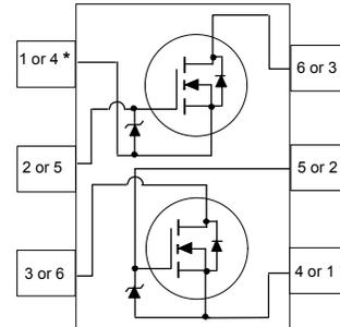
\* The pinouts are symmetrical; pin 1 and 4 are interchangeable.
