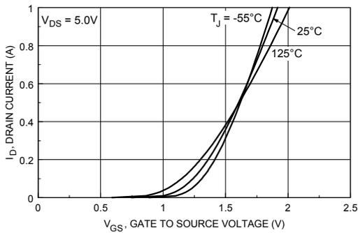
Figure 5. Transfer Characteristics.
