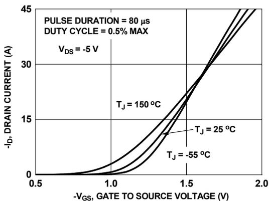
**Figure 5. Transfer Characteristics**
