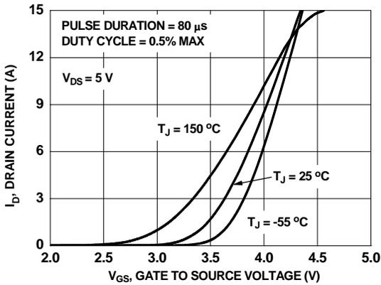
Figure 5. Transfer Characteristics
