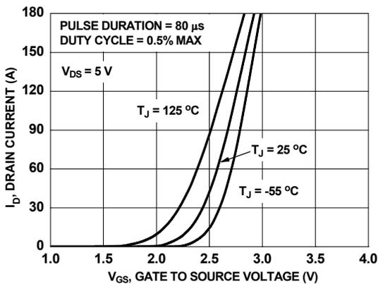
**Figure 5. Transfer Characteristics**
