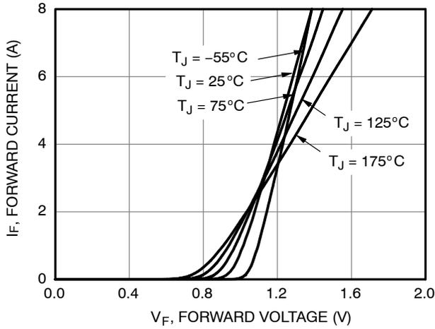
Figure 1. Forward Characteristics
