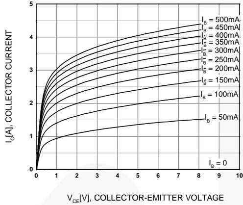
Figure 1. Static Characteristic
