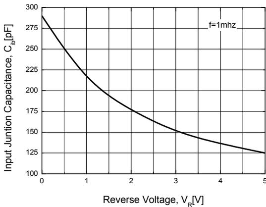
**Figure 11. Input Capacitance**
