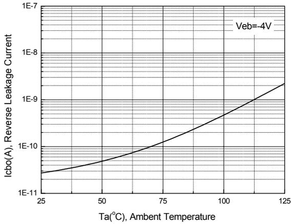
**Figure 9. Base-Emitter Leakage Current**
