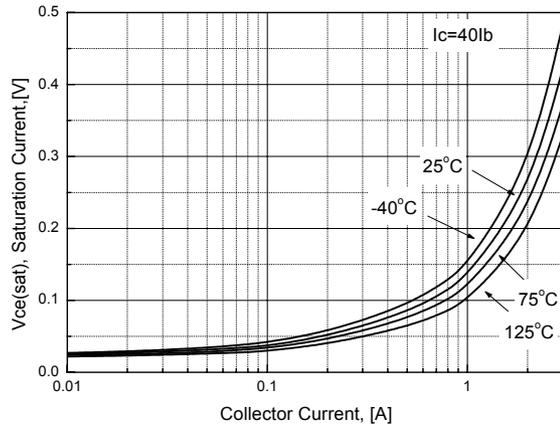
**Figure 4. Collector-Emitter Saturation Voltage(1)**
