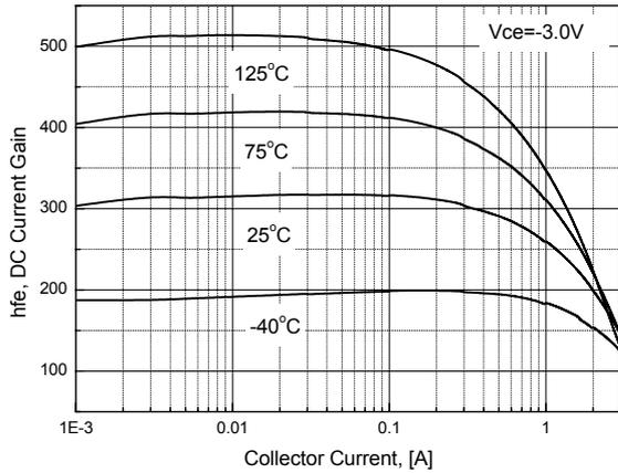
**Figure 3. DC Current Gain, Vce=3V**
