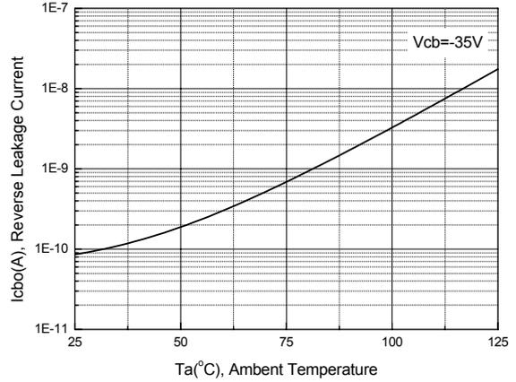
**Figure 8. Collector-Base Leakage Current**
