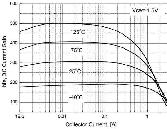
**Figure 1. DC Current Gain, Vce=1.5V**
