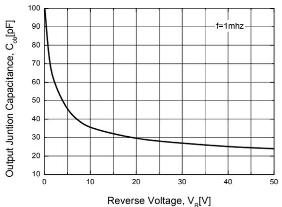
**Figure 12. Output Capacitance**
