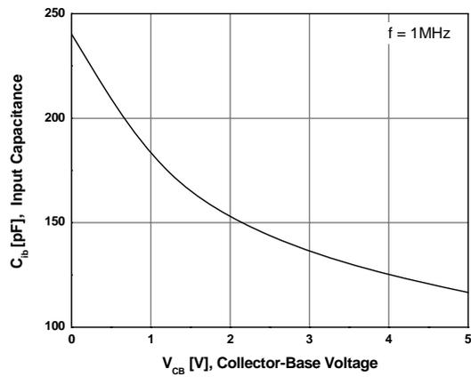
**Figure 8. Input Capacitance**
