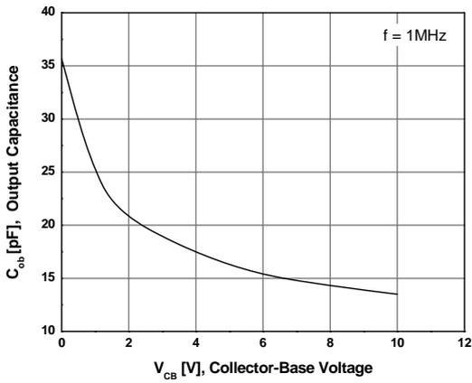
**Figure 7. Output Capacitance**
