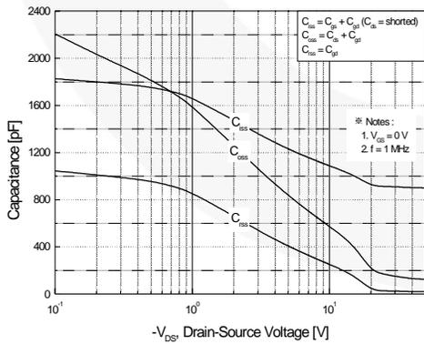
Figure 5. Capacitance Characteristics
