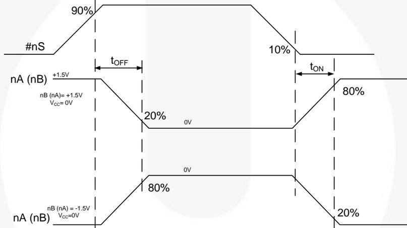
**Figure 5.  $t_{ON}/t_{OFF}$  Select (#nS) to Output Timing**
