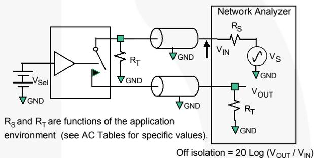
**Figure 16. Channel-Off Isolation**
