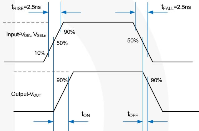
**Figure 11. Turn-On / Turn-Off Waveforms**
