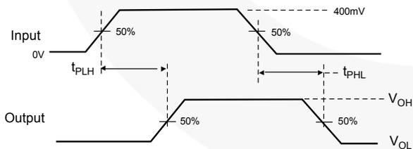
**Figure 12. Propagation Delay ( $t_{rtf} = 500ps$ )**
