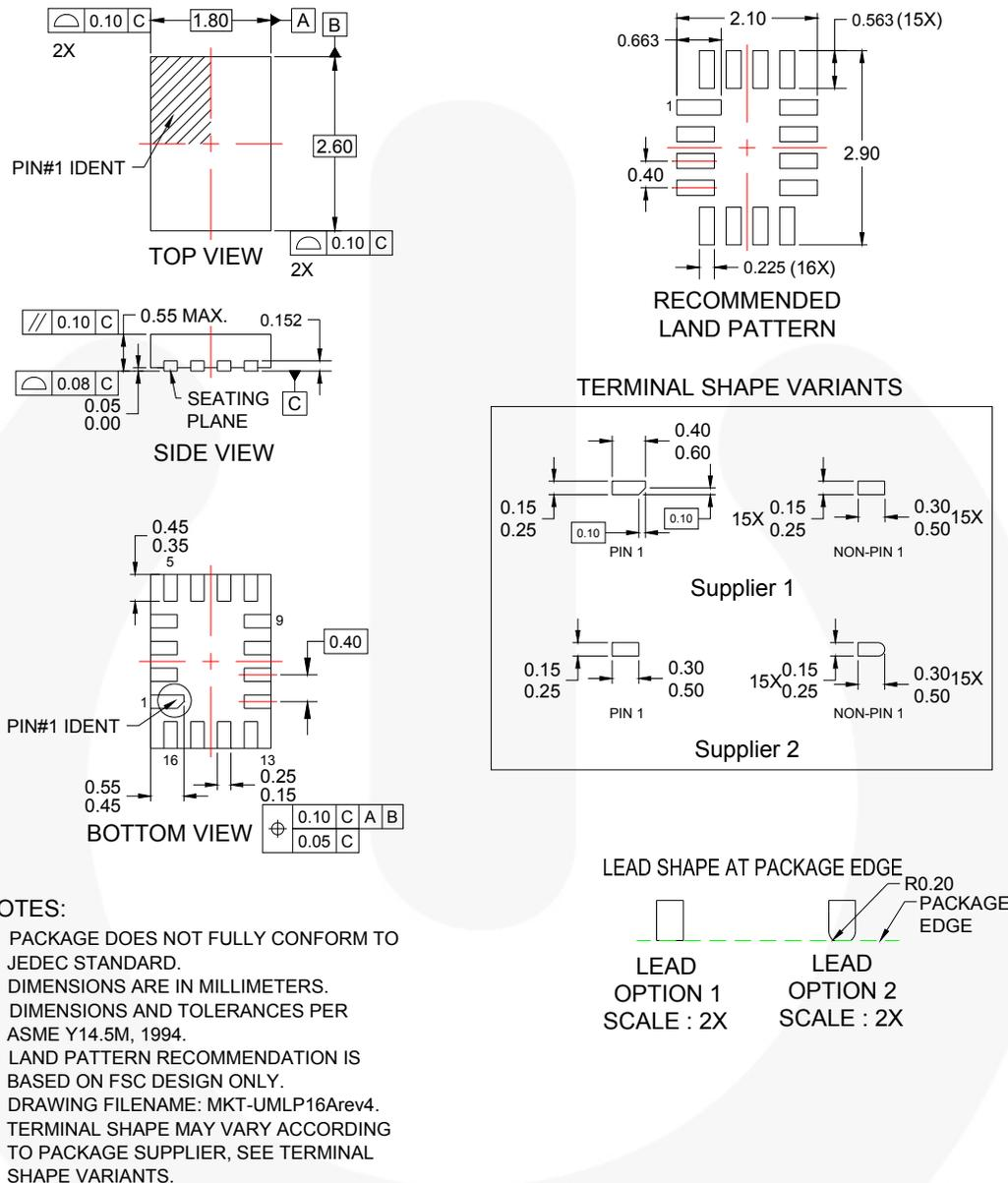
**Figure 20. 16-Pin Ultrathin Molded Leadless Package (UMLP)**
