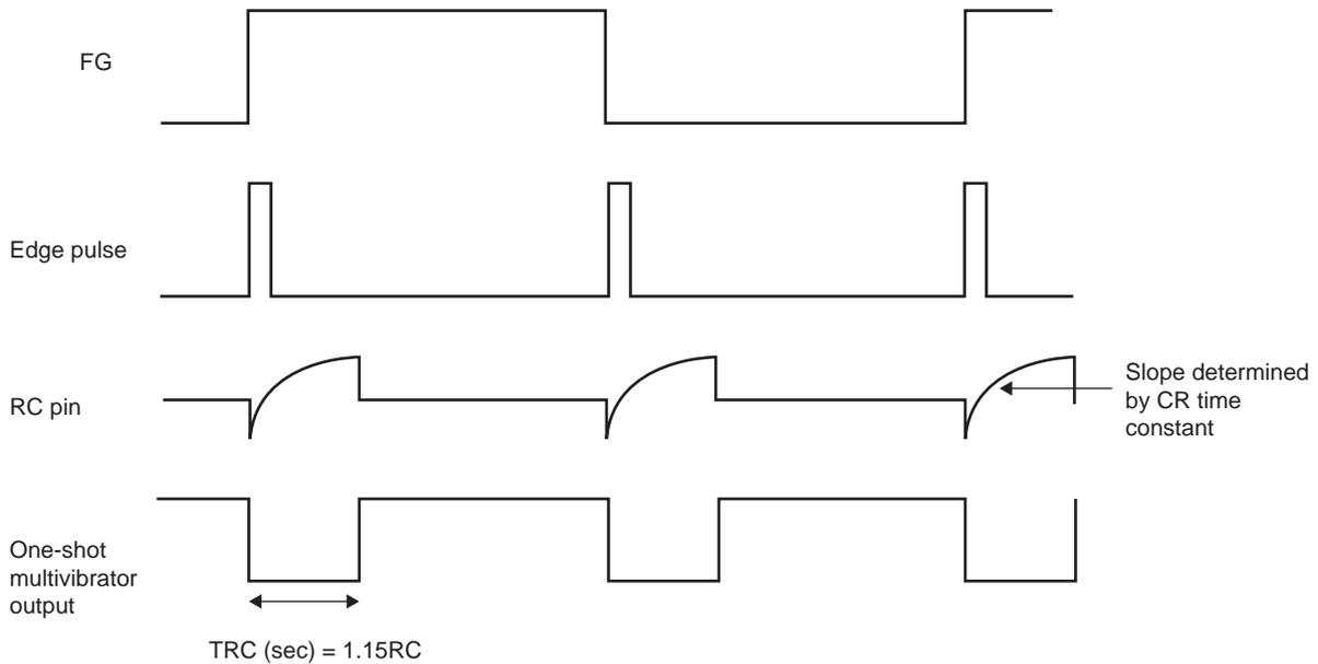
By changing the pulse width as determined by the CR time constant, the VCTL versus rotational speed slope can be adjusted as shown in the speed control diagram in the previous section.
