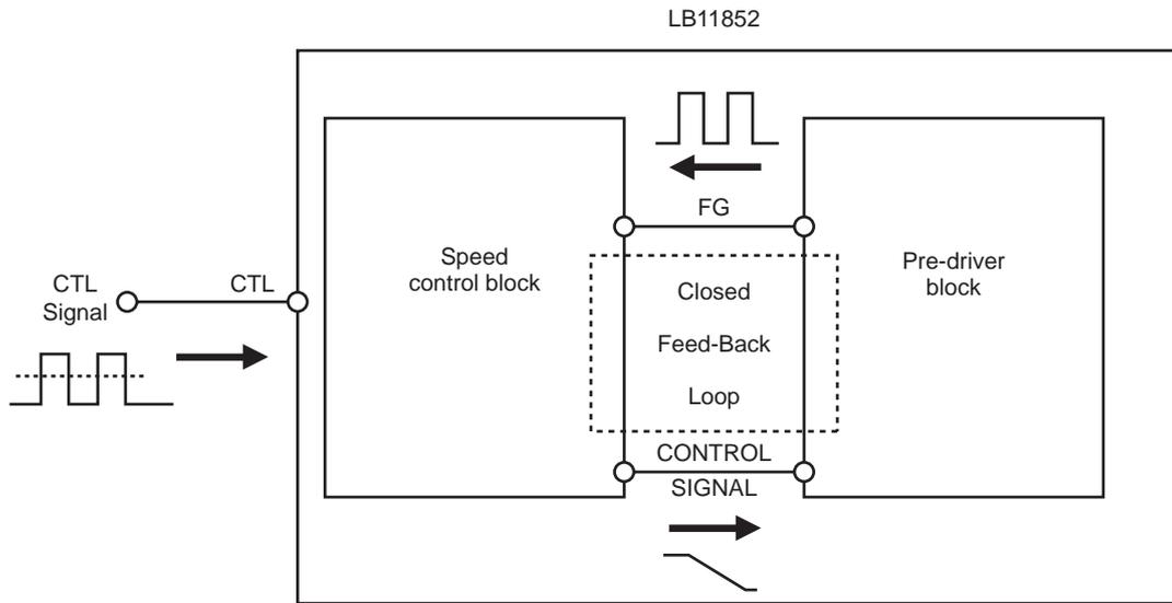
The operation inside the IC is as follows. Pulse signals are created from the edges of the FG signals as shown in the figure below, and using these signals as a reference, waveforms with a pulse width determined by the CR time constant are generated using a one-shot multivibrator. These pulse waveforms are then integrated to control the duty ratio of the pre-driver output as the control voltage.
