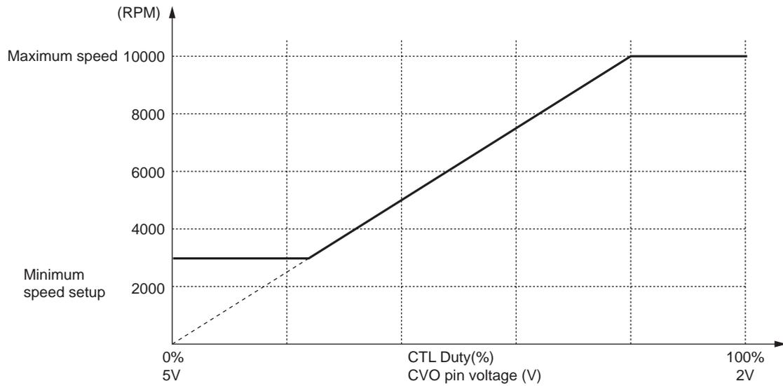
1) Obtain the ratio of the minimum speed required to the maximum speed.
