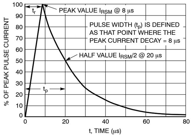
**Figure 2. 8 X 20  $\mu\text{s}$  Pulse Waveform**
