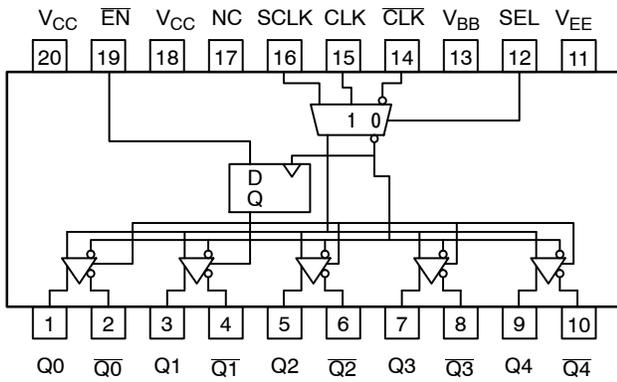
Warning: All  $V_{CC}$  and  $V_{EE}$  pins must be externally connected to Power Supply to guarantee proper operation.
