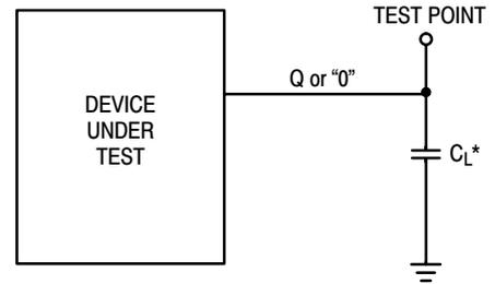
\*Includes all probe and jig capacitance.
