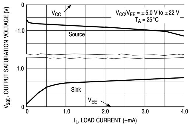
**Figure 3. Split Supply Output Saturation versus Load Current**
