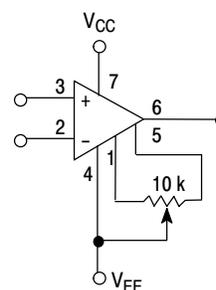
Offset Nulling range is approximately  $\pm 80 \text{ mV}$  with a 10 k potentiometer, MC33171 only.
