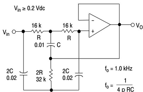
Figure 14. Active High-Q Notch Filter
