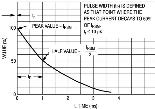
Figure 5. 10 × 1000 µs Pulse Waveform
