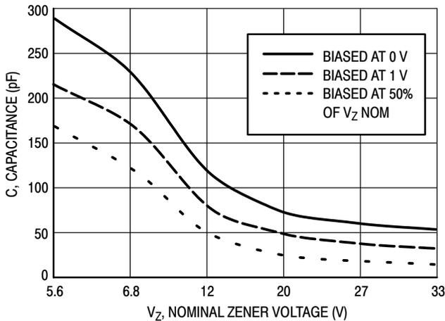
Figure 1. Typical Capacitance
