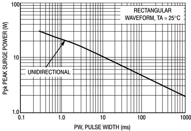
Figure 7. Maximum Non-Repetitive Surge Power, Ppk versus PW
