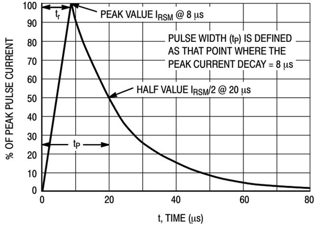
Figure 6. 8 × 20 µs Pulse Waveform
