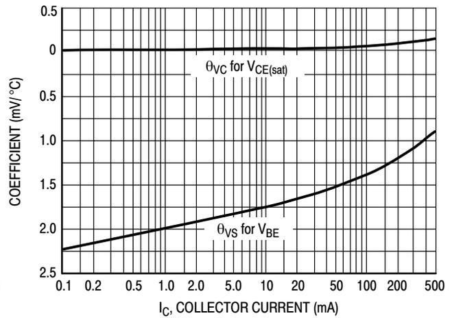
Figure 17. Temperature Coefficients
