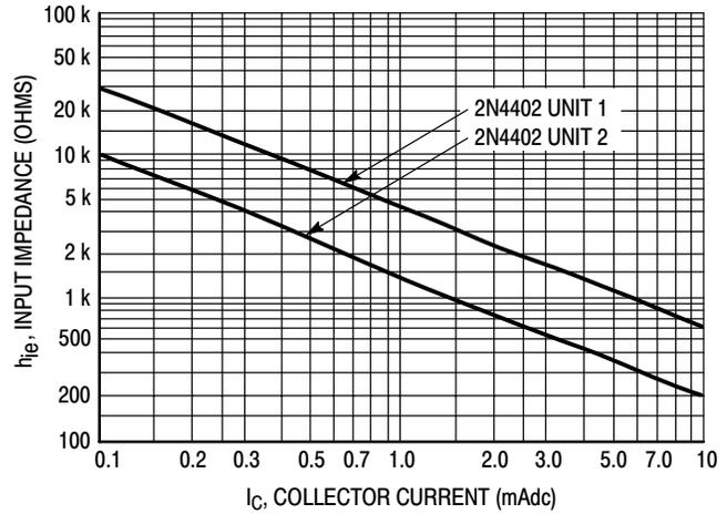
Figure 11. Input Impedance
