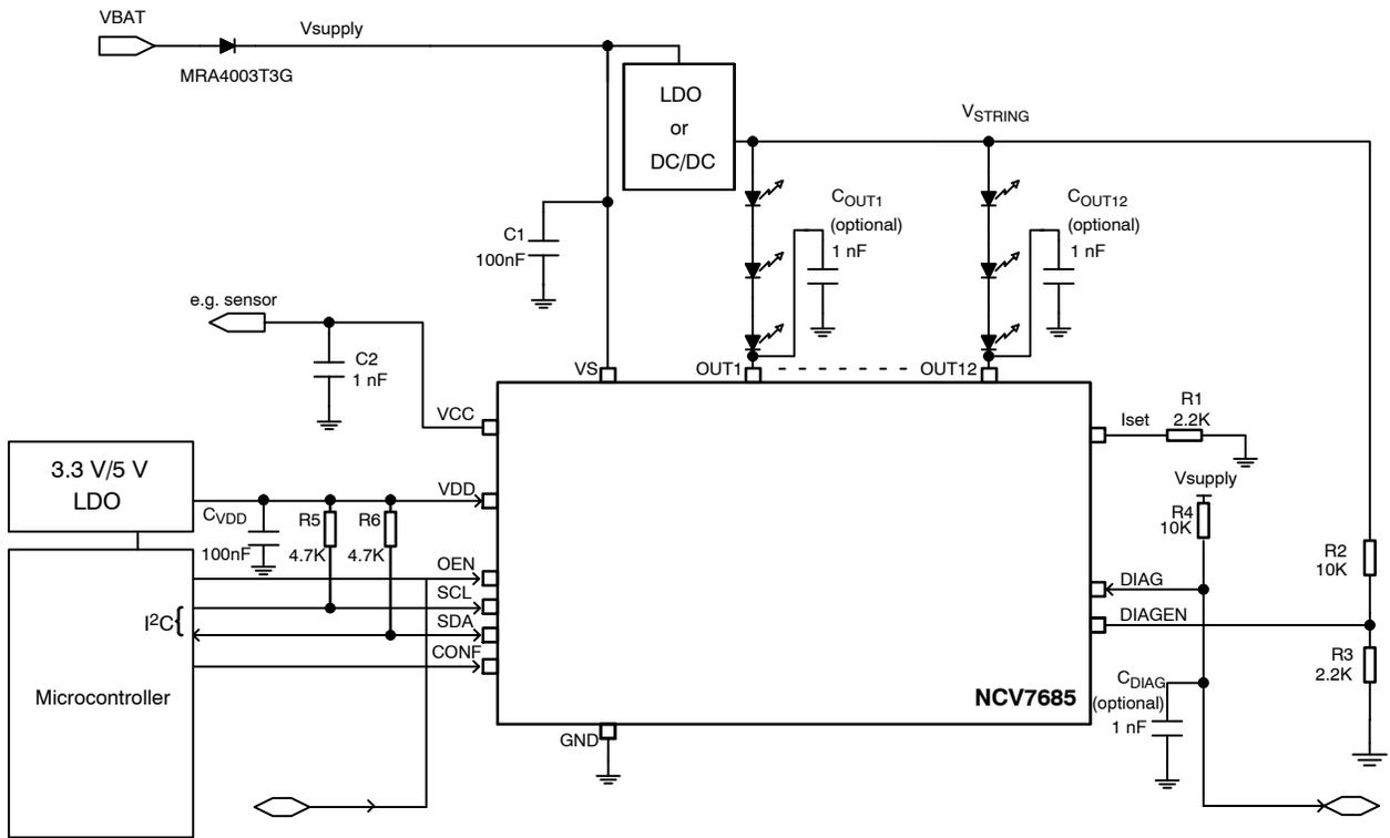
Figure 3. Application Diagram with Micro-controller (I<sup>2</sup>C Mode)
