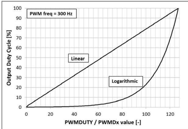
Figure 11. Output Duty Cycle vs. Register Setting
