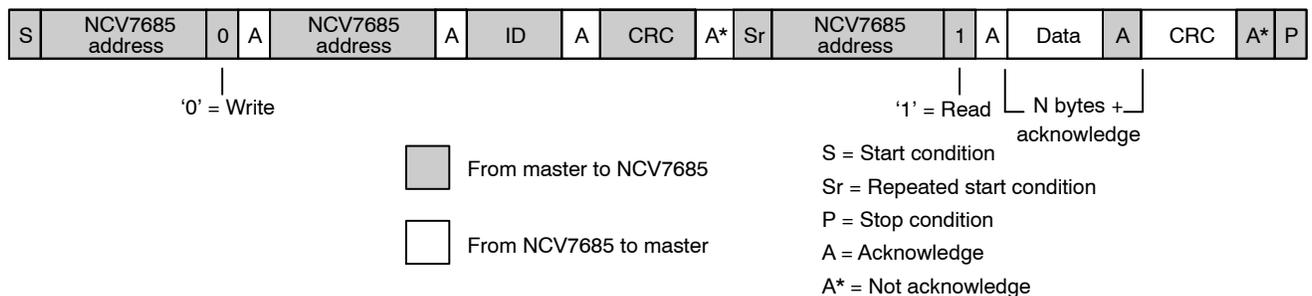
**Figure 8. Format of I2C Read Access Frames**
