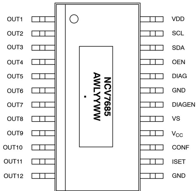
Figure 2. Pinout Diagram
