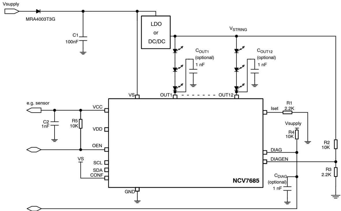
Figure 4. Application Diagram without Micro-controller (Stand Alone Mode)
