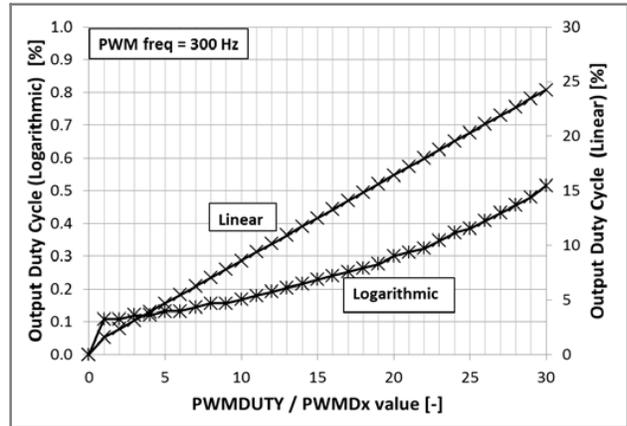
Figure 12. Output Duty Cycle vs. Register Setting - Detail
