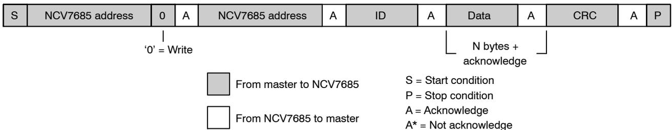
**Figure 7. Format of I2C Write Access Frames**
