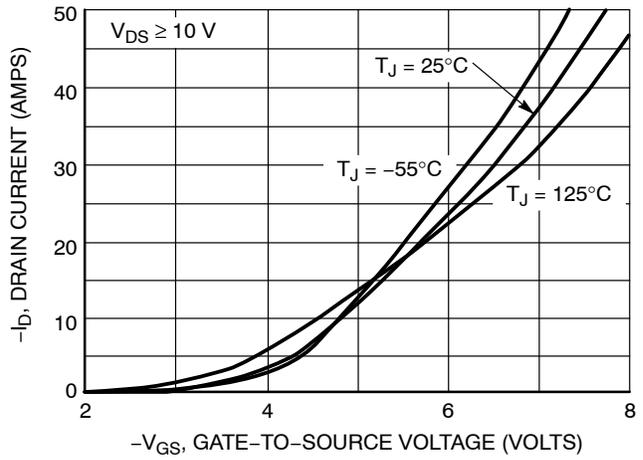
**Figure 2. Transfer Characteristics**
