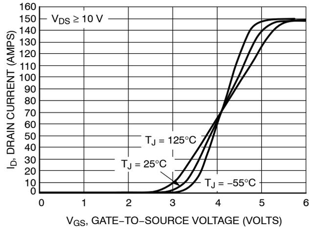
Figure 2. Transfer Characteristics
