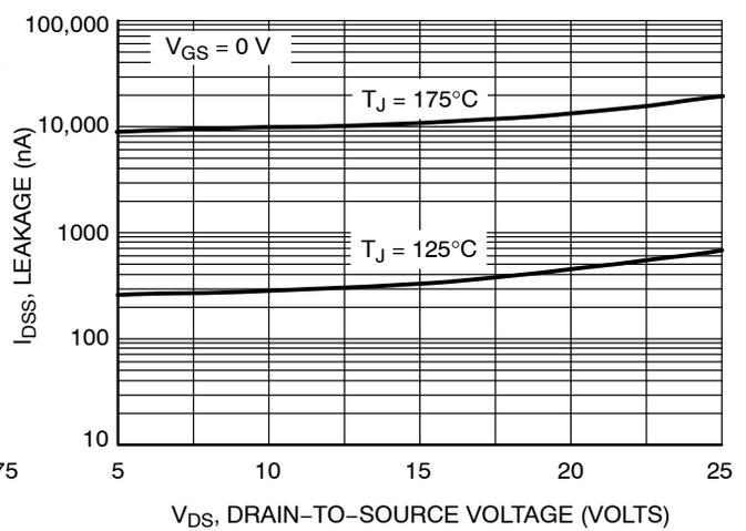
Figure 6. Drain-to-Source Leakage Current vs. Drain Voltage
