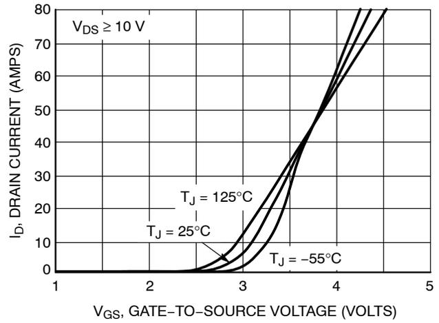
**Figure 2. Transfer Characteristics**
