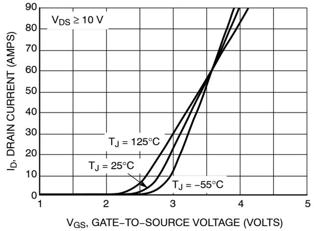
Figure 2. Transfer Characteristics
