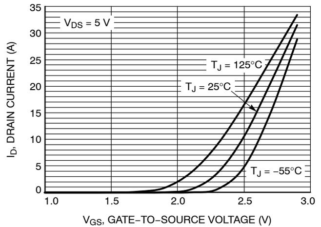
Figure 2. Transfer Characteristics
