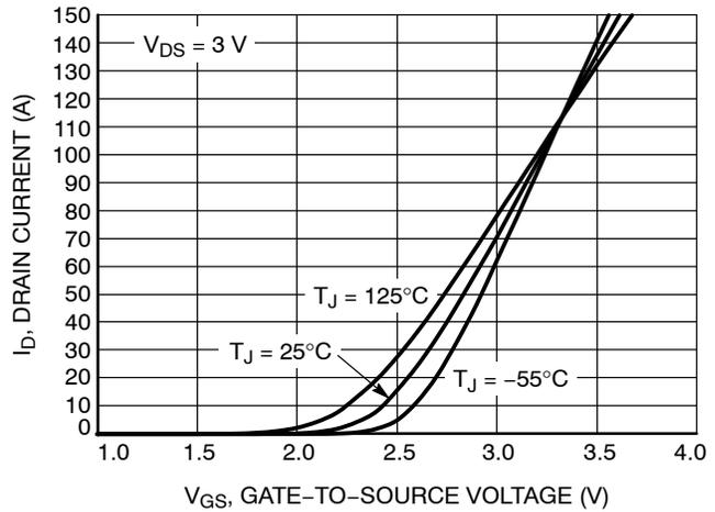
Figure 2. Transfer Characteristics
