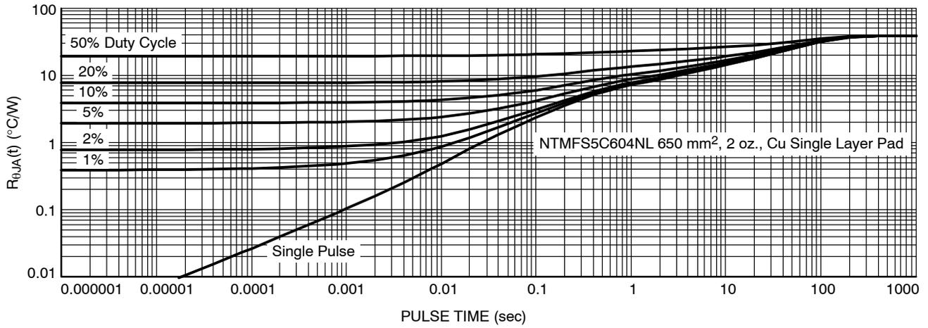
Figure 13. Thermal Characteristics
