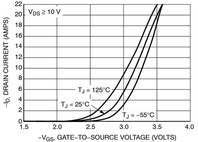
Figure 2. Transfer Characteristics
