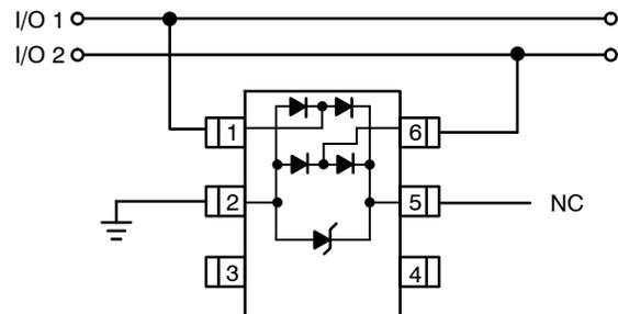
In applications lacking a positive supply reference or those cases in which a fully isolated power supply is required, the internal surge protection can be used as the reference. For these applications, pin 5 is not connected. In this configuration, the steering diodes will conduct whenever the voltage on the protected line exceeds the working voltage of the surge protection plus one diode drop ( $V_c = V_f + V_{RWM}$ ).
