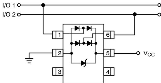
For this configuration, connect pin 5 directly to the positive supply rail ( $V_{CC}$ ), the data lines are referenced to the supply voltage. The internal surge protection diode prevents overvoltage on the supply rail. Biasing of the steering diodes reduces their capacitance.
