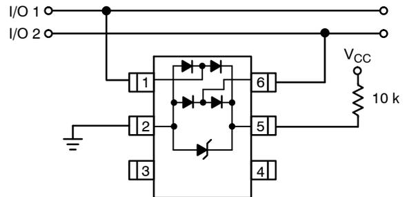
The NUP2201MR6 can be isolated from the power supply by connecting a series resistor between pin 5 and  $V_{CC}$ . A 10 kΩ resistor is recommended for this application. This will maintain bias on the internal surge protection and steering diodes, reducing their capacitance.
