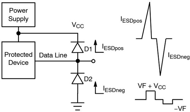
Looking at the figure above, it can be seen that when a positive ESD condition occurs, diode D1 will be forward biased while diode D2 will be forward biased when a negative ESD condition occurs. For slower transient conditions, this system may be approximated as follows:
