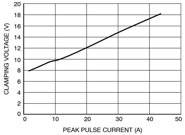
Figure 8. Clamping Voltage vs. Peak Pulse Current
