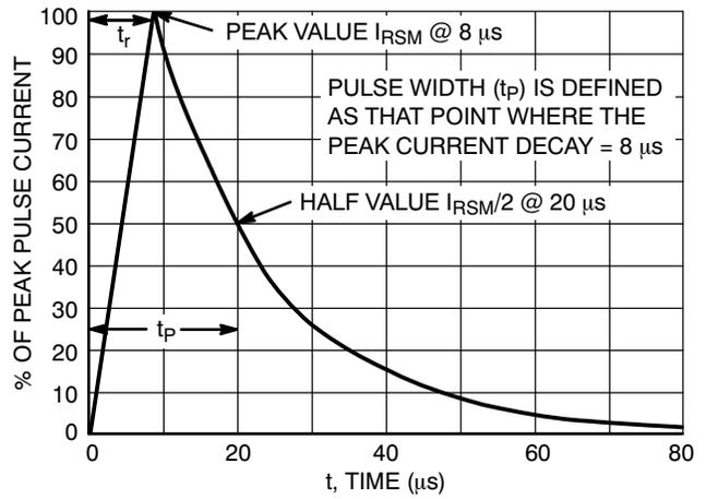
Figure 4.  $8 \times 20 \mu\text{s}$  Pulse Waveform
