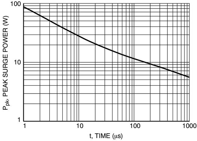
Figure 1. Pulse Width
