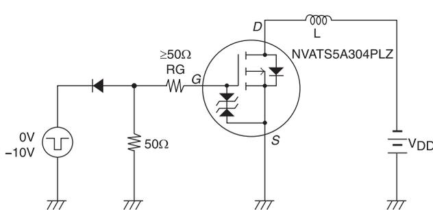
Fig.2 Switching Time Test Circuit
