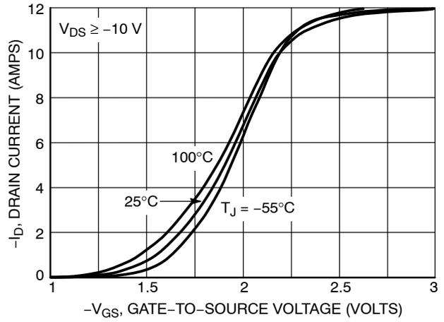
Figure 2. Transfer Characteristics
