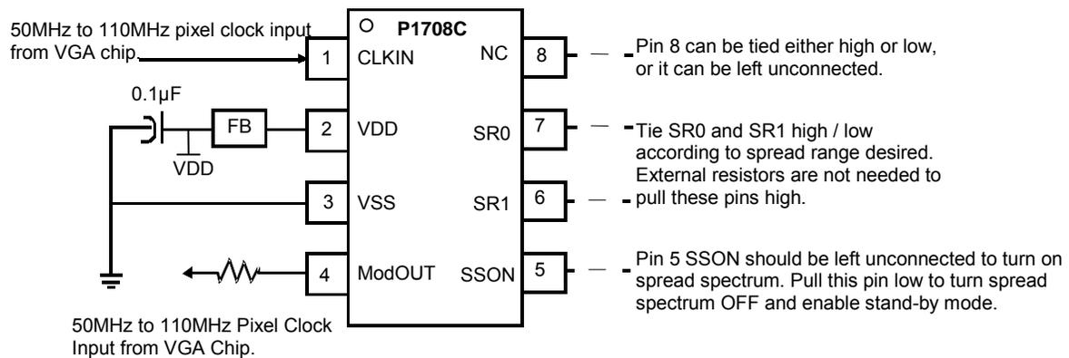
**Note:** To set the P1708C to standby mode, disable the input clock (pin 1 CLKIN) and pull SSON (pin 5) low. Refer to *Standby Mode Selection Table*.
